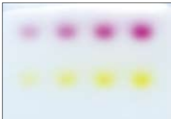
Fig. 1. RubyTaq™ DNA Polymerase visualization during gel electrophoresis. RubyTaq in PCR does not require the use of additional loading buffer. Simply load onto an agarose gel directly after cycling. During electrophoresis, RubyTaq separates into 2 colors, magenta (runs between 500 bp [2% gels] and 1500 bp [0.8% gels]) and yellow (runs less than 10 bp). The indicated volumes of RubyTaq DNA Polymerase were run on a 1% TAE agarose gel.
